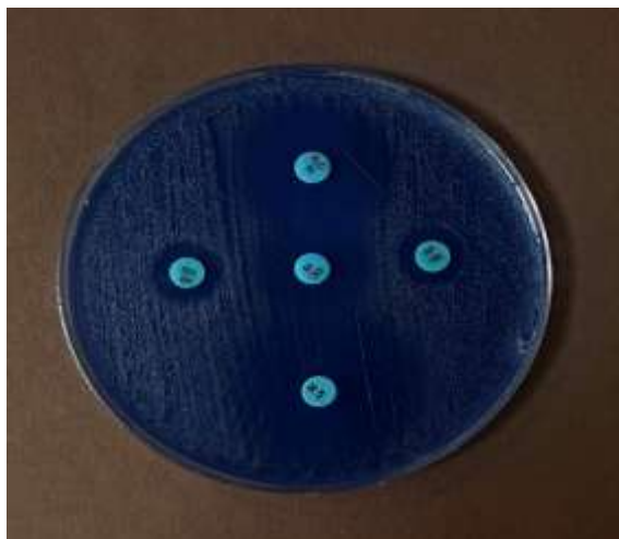
Figure 1: Antifungal susceptibility testing by Kirby Bauer disc diffusion method.
