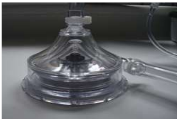
Figure 2: Blood centrifugal pump with stacked cones. [20]
